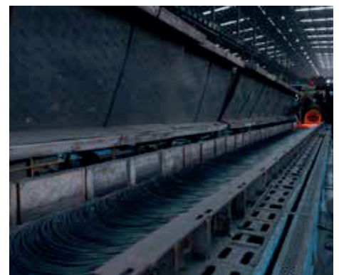
Controlled Cooling Conveyor The cooling capability of this conveyor enables the production of high-medium carbon and boron alloy wire rods for required structure and hardness.
