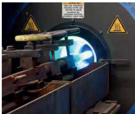
Surface Imperfections Detector Surface imperfections are controlled throughout the wire rod to guarantee proper surface quality.
